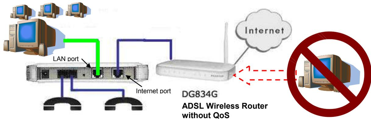
*Note: If you encounter problems using this method you may need to enable the DMZ option of the ADSL/CABLE/WIRELESS ROUTER and point it to the IP address assigned to the NETGEAR VoIP device. Alternatively you should port forward the following ports to the NETGEAR VoIP device;*
